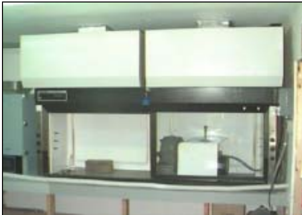
Grinding of soil sample is performed under the fume hood, which exhausts to the HEPA filter.
