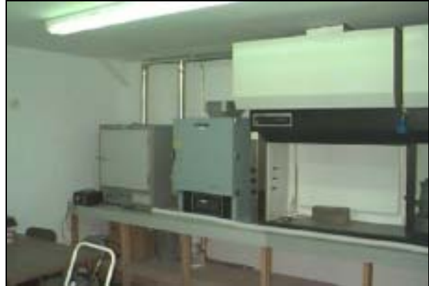
Electric ovens are used to dry the soil samples prior to grinding.
