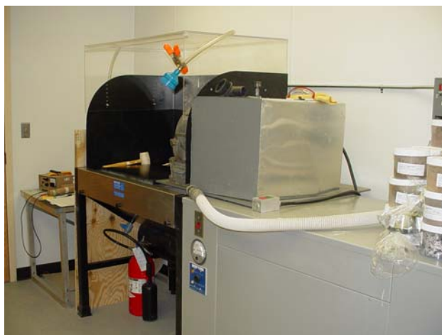
View of downdraft table and adjacent unit containing the High Efficiency Particulate Air (HEPA) filter.
