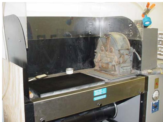
The downdraft table and pulverizer in the Soil Preparation Laboratory.
