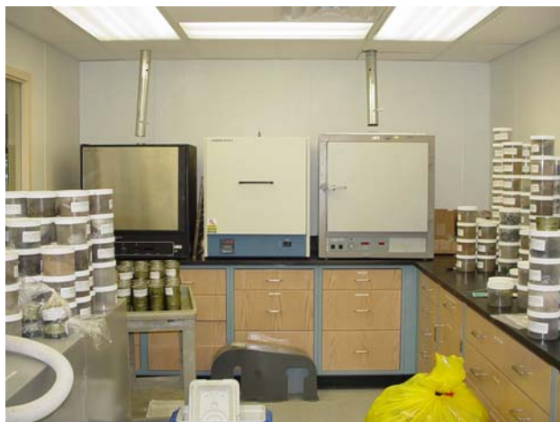
Soil Preparation Laboratory. View of the vented drying ovens and muffle furnace (center).
