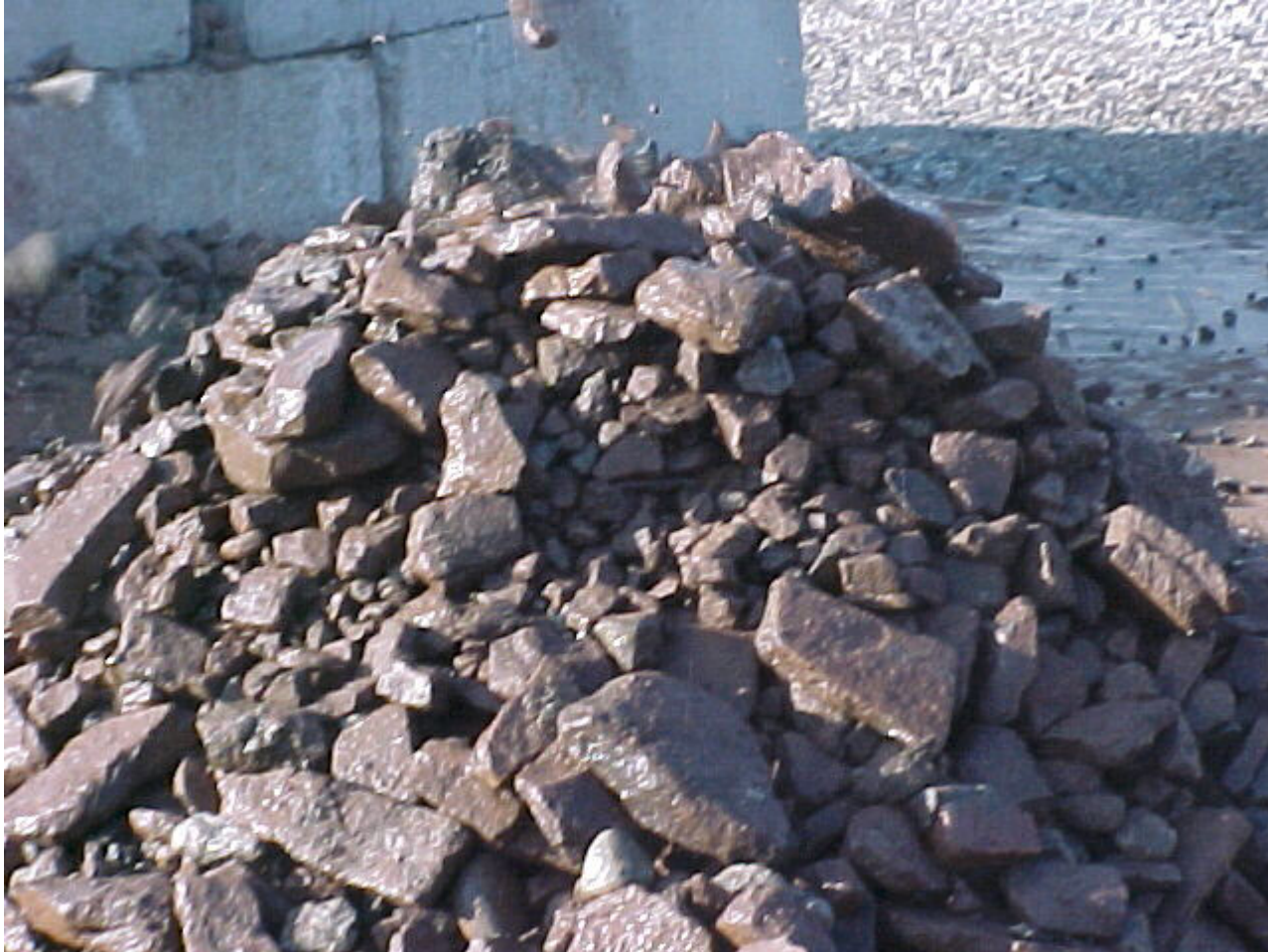
Rinsed Product with one pass through the Gravel Separation System utilizing Recycled Water
