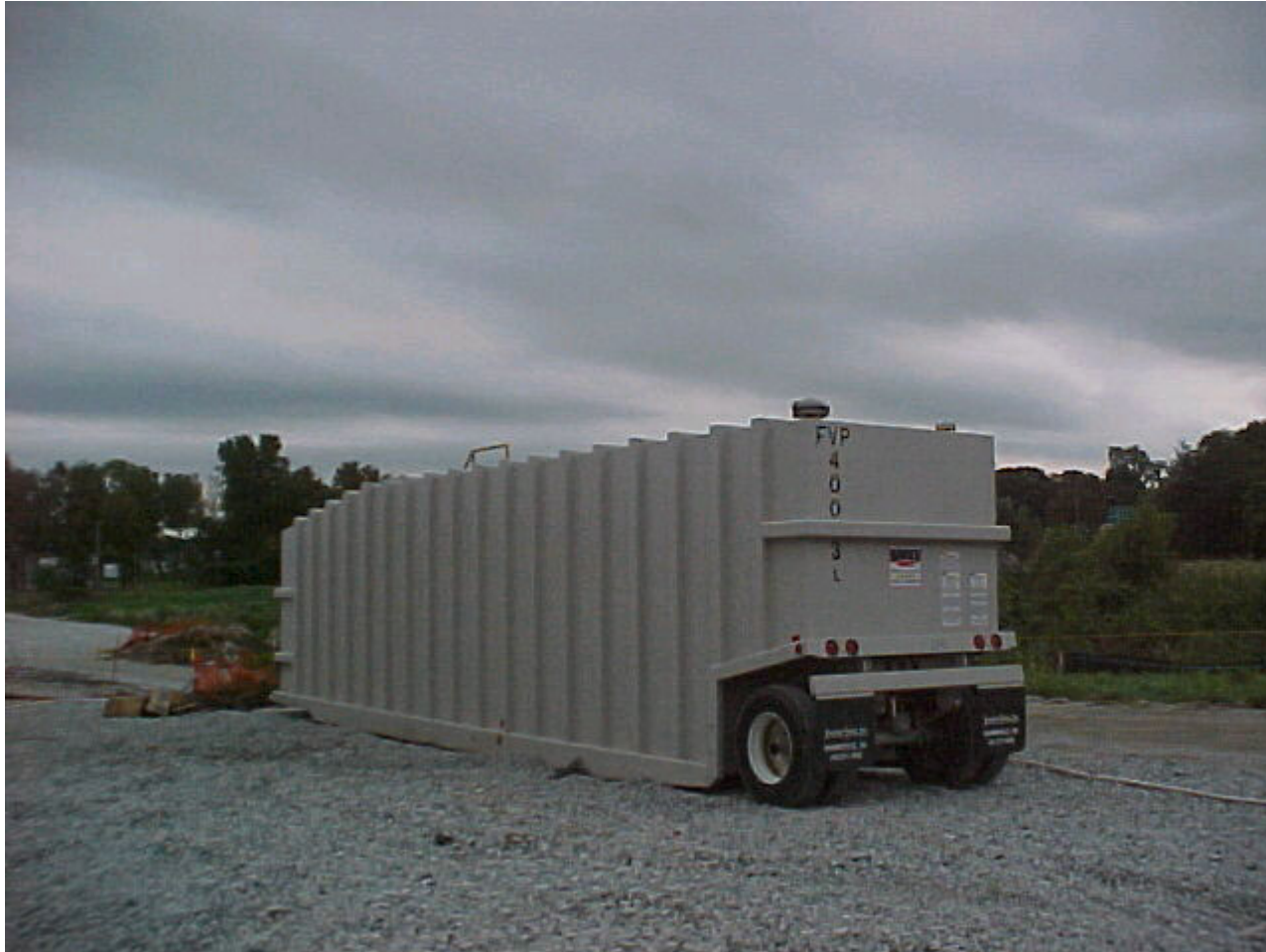
20,000 Gallon Capacity for Water Storage and Re-cycle for the Rinse Unit
