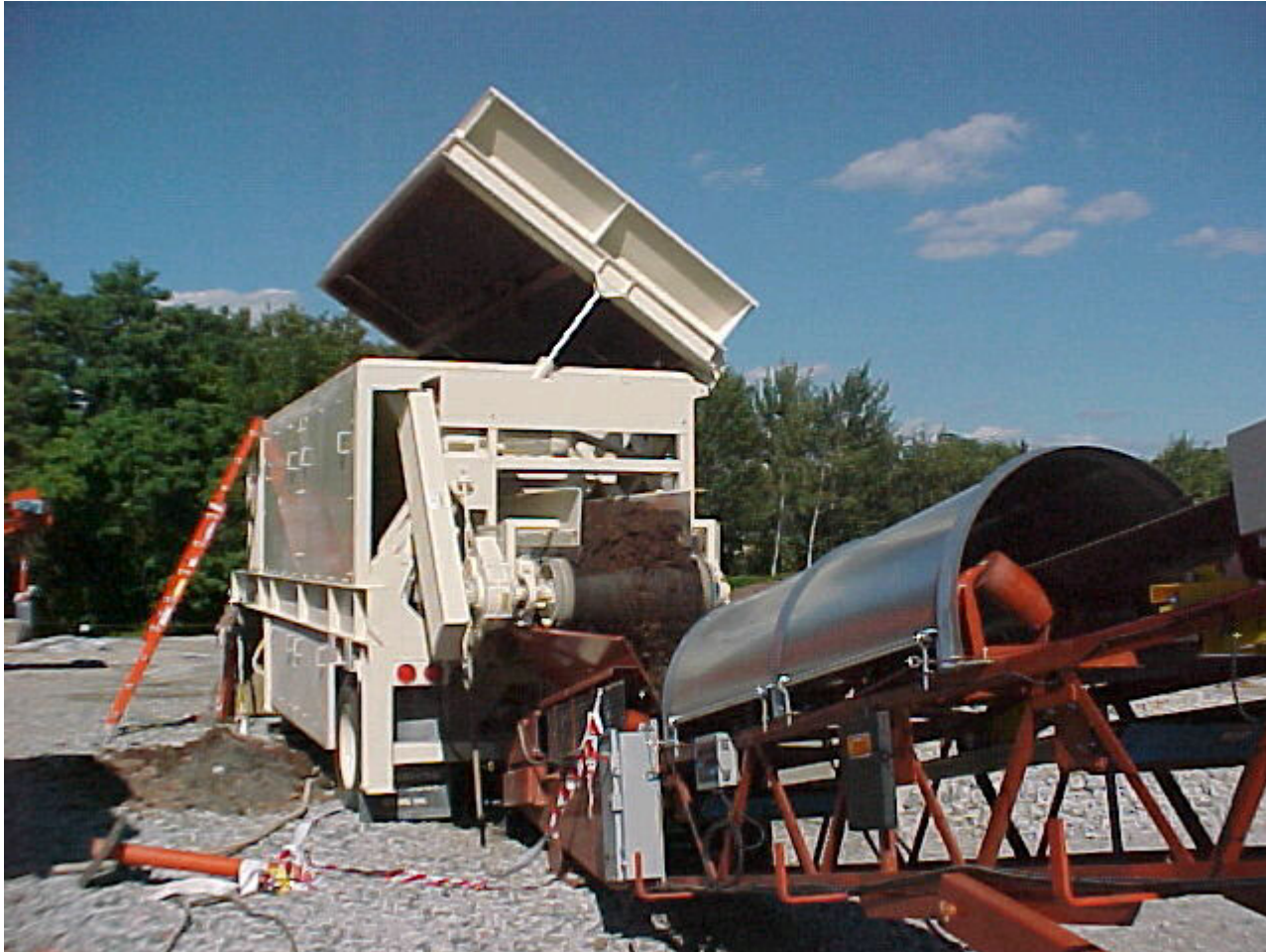
Temporary Grizzly and Hopper Set-up - Direct Feed to the Radiological Sorting System
