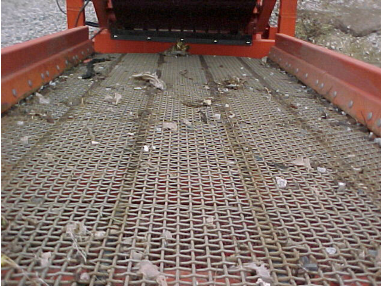
Gravel Separation System - Top Screen Deck
