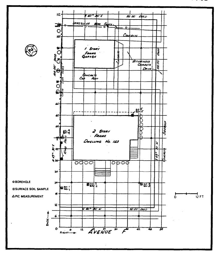
FIGURE 2-1 LOCATIONS OF BOREHOLES, SOIL SAMPLES, AND PIC MEASUREMENTS AT 123 AVENUE F
