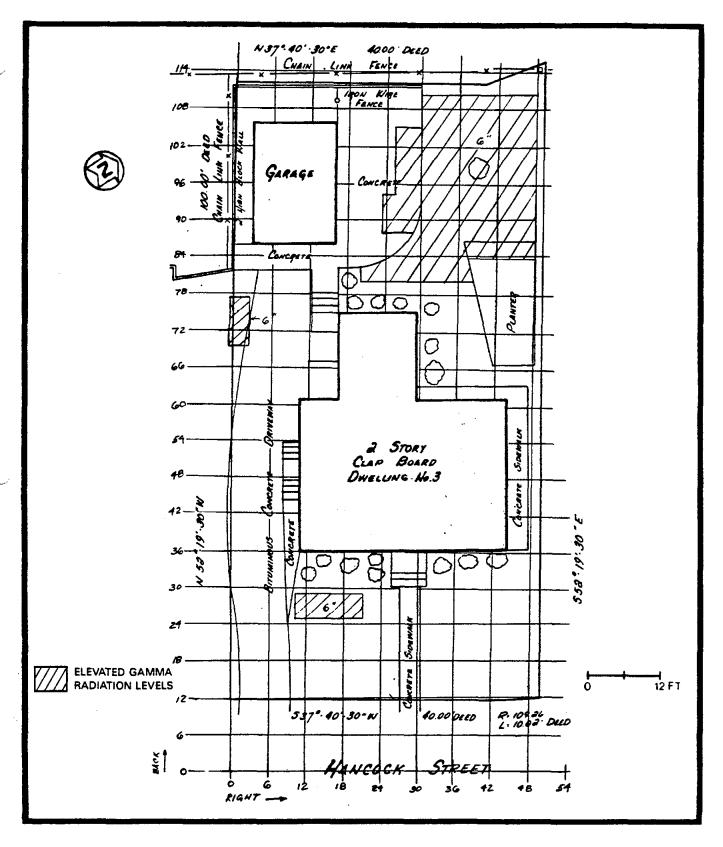
FIGURE 3-1 AREAS OF ELEVATED GAMMA RADIATION LEVELS AT 3 HANCOCK STREET
