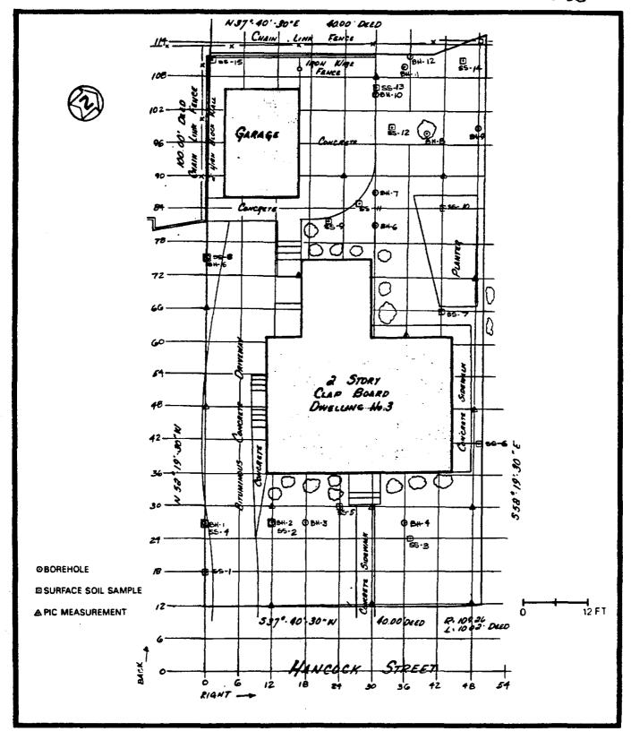
FIGURE 2-1 LOCATIONS OF BOREHOLES, SOIL SAMPLES, AND PIC MEASUREMENTS AT 3 HANCOCK STREET
