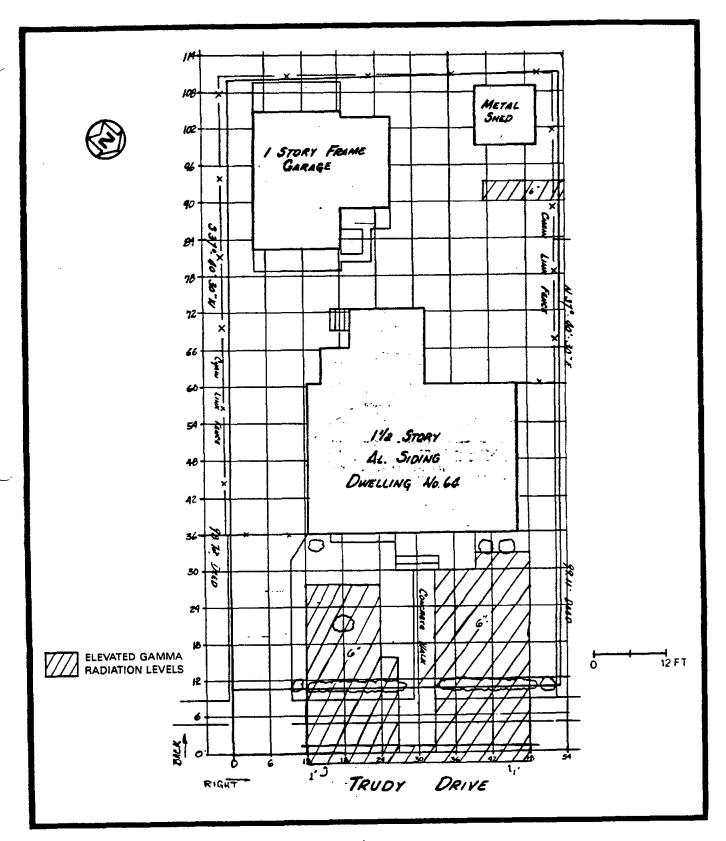
FIGURE 3-1 AREAS OF ELEVATED GAMMA RADIATION LEVELS AT 64 TRUDY DRIVE
