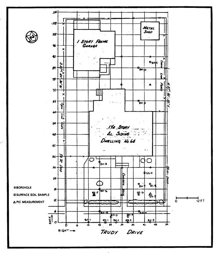
FIGURE 2-1 LOCATIONS OF BOREHOLES, SOIL SAMPLES, AND PIC MEASUREMENTS AT 64 TRUDY DRIVE
