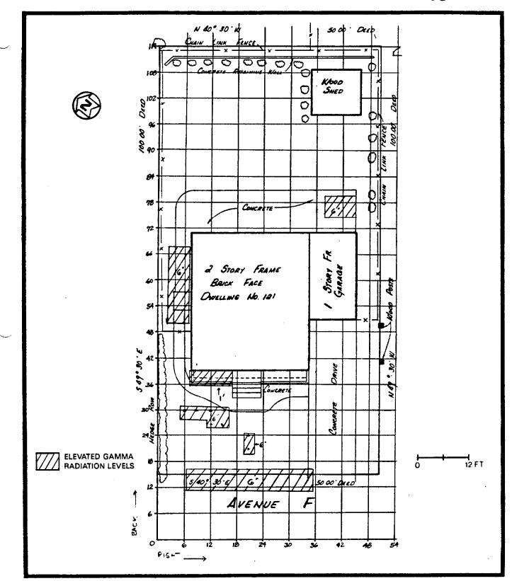
FIGURE 3-1 AREAS OF ELEVATED GAMMA RADIATION LEVELS AT 121 AVENUE F
