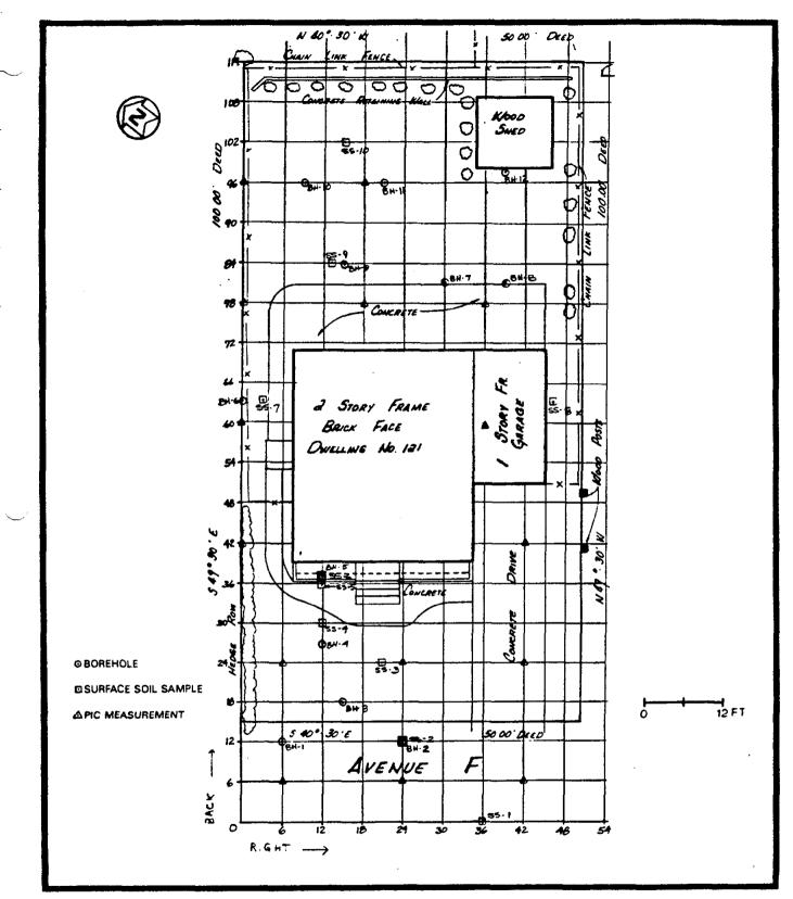
FIGURE 2-1 LOCATIONS OF BOREHOLES, SOIL SAMPLES, AND PIC MEASUREMENTS AT 121 AVENUE F
