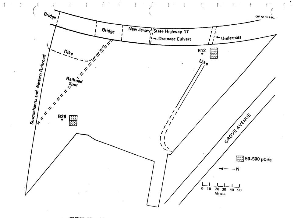
FIGURE 13. Plan View With Subsurface Th-232 Concentrations Indicated for Boreholes B12 and B26.
