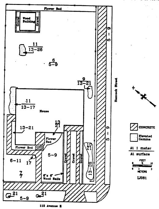
Fig. 1. Gamma radiation levels ( $\mu$ R/h) measured on the surface at 113 Avenue E, Lodi, New Jersey (LJ081), with corresponding measurements one meter above the surface where indicated.
