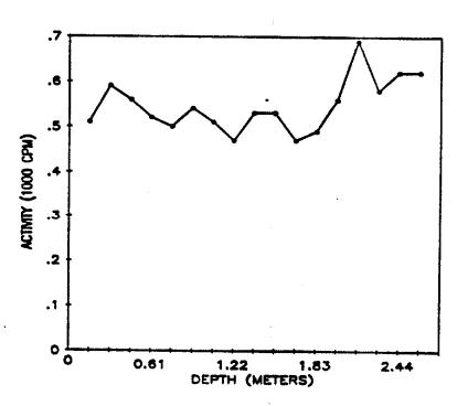
Fig. 3. Gamma profile for auger hole 1 (LJ072A1) at 160 Essex Street, Lodi, New Jersey.
