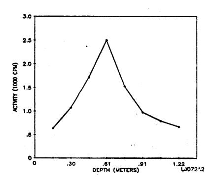
Fig. 4. Gamma profile for auger hole 2 (LJ072A2) at 160 Essex Street, Lodi. New
