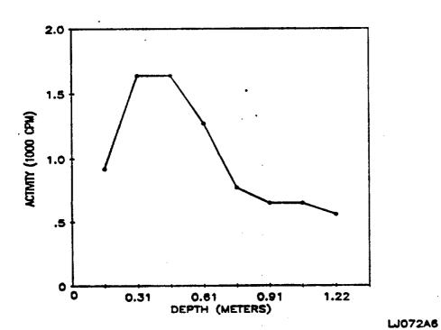
Fig. 8. Gamma profile for auger hole 6 (LJ072A6) at 160 Essex Street, Lodi, New Jersey.
