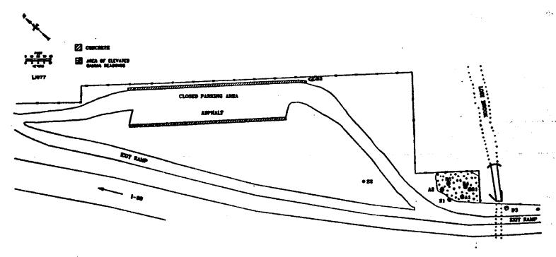
Fig. 2. Diagram showing locations of soil samples taken at Interstate 80, North Right of Way at Lodi Brook, Lodi, New Jersey (LJ077).
