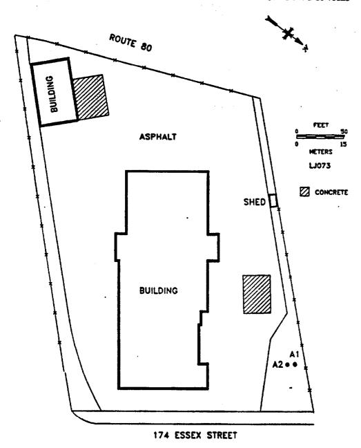
Fig. 2. Diagram showing locations of soil samples taken at 174 Essex Street, Lodi, New Jersey (LJ073).
