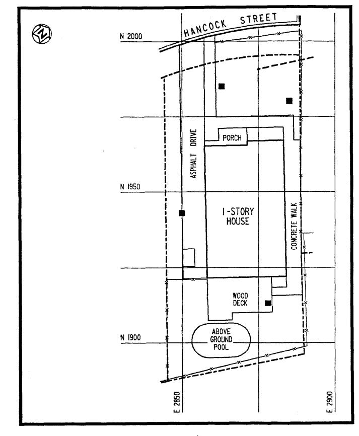
FIGURE 4-3 GAMMA EXPOSURE RATE MEASUREMENT LOCATIONS AT 10 HANCOCK STREET
