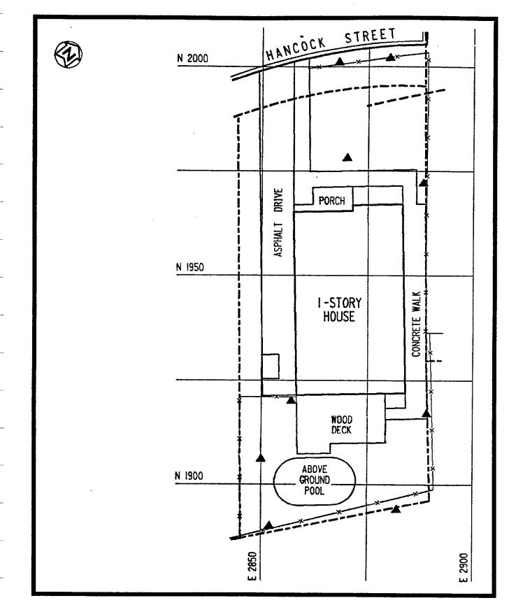
FIGURE 4-2 SURFACE AND SUBSURFACE SOIL SAMPLING LOCATIONS AT 10 HANCOCK STREET
