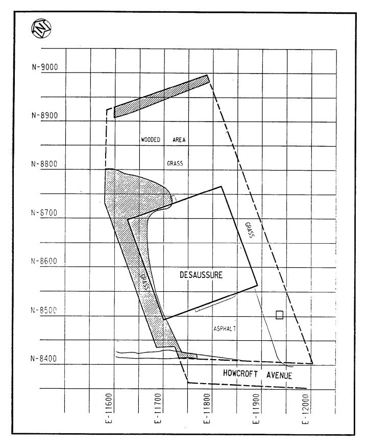
FIGURE 5-2 AREAS OF SUBSURFACE CONTAMINATION AT DESAUSSURE
