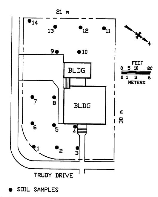
Fig. 4. Locations of soil samples on the property at 58 Trudy Drive, Lodi, New Jersey (LN001V).
