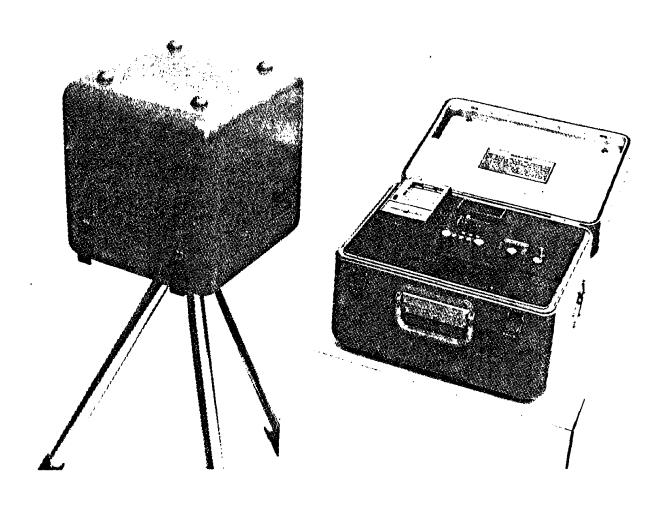
Fig. I-E. Pressurized Ion Chamber.
