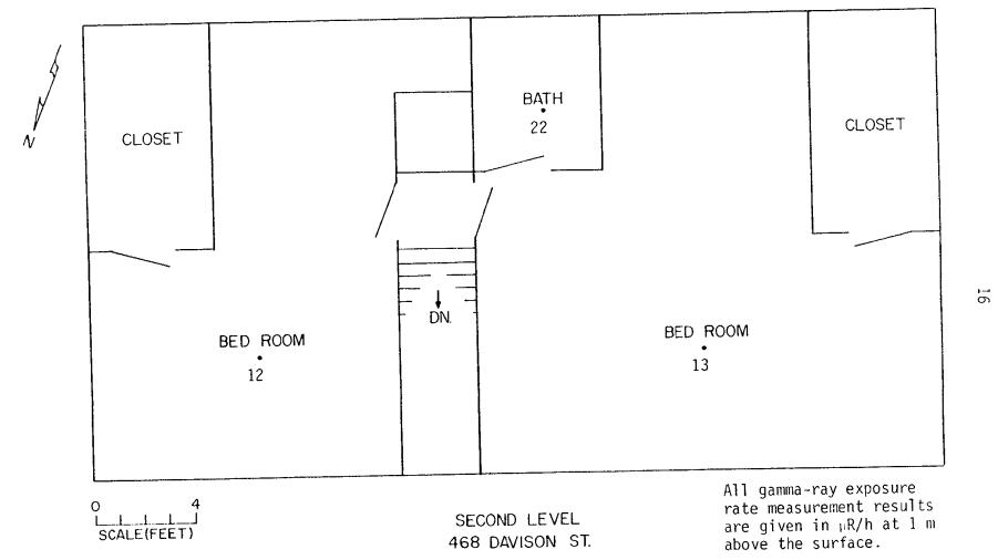
Fig. 8. Schematic of the second level floor plan at 468 Davison Avenue showing external gamma-ray measurement results
