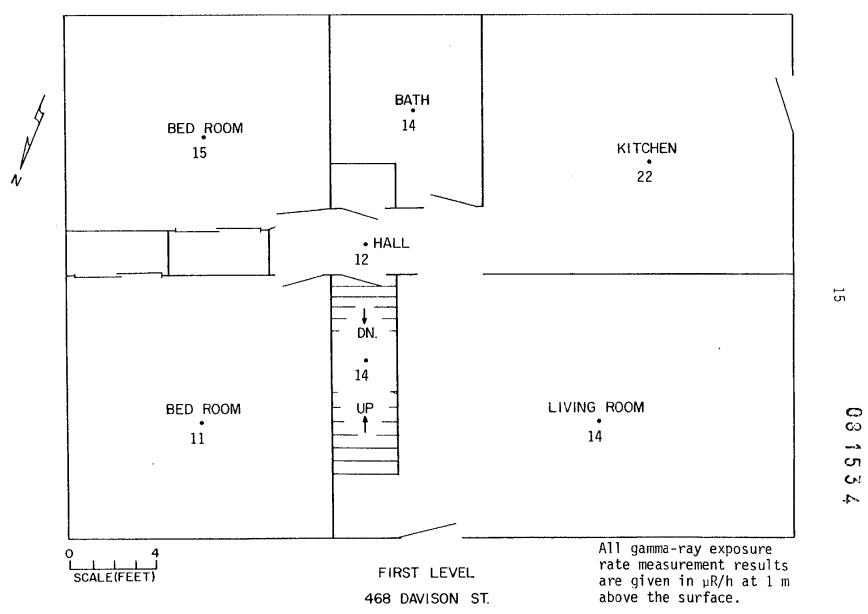
Fig. 7. Schematic of the first level floor plan at 468 Davison Avenue
