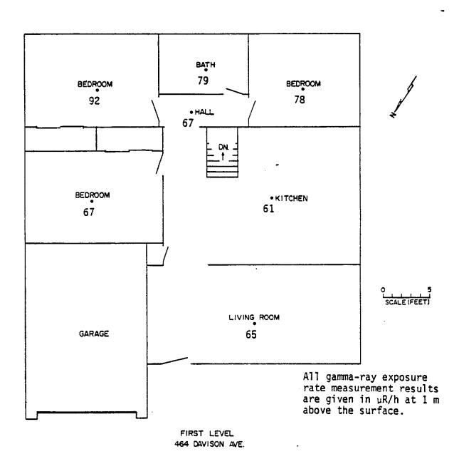
g. 7. Schematic of the first level floor plan at 464 Davison Avenue showing external gamma-ray measurement results.
