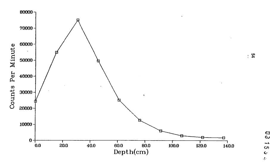
Fig. II-11. Gamma profile of core hole MJC29 (see Fig. 6)
