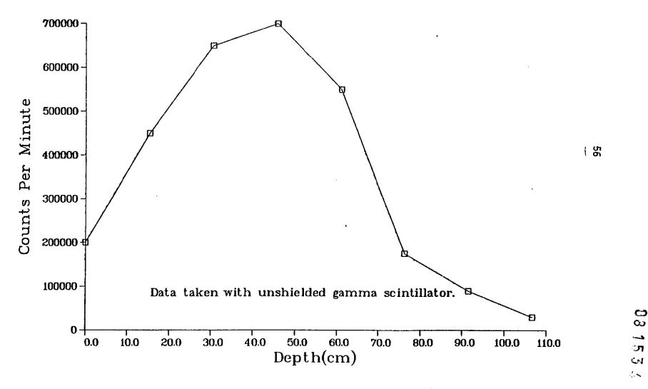
Fig. II-13. Gamma profile of core hole MJC31 (see Fig. 8)
