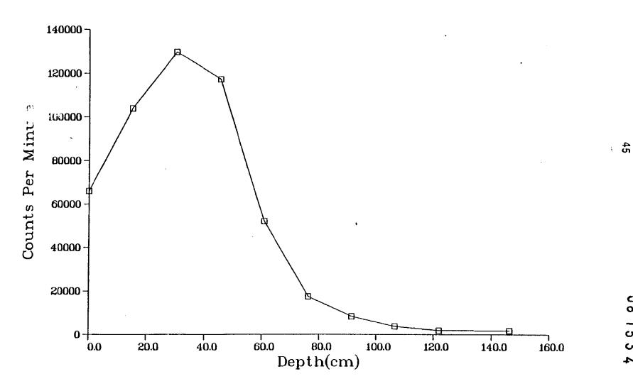
Fig. II-2. Gamma profile of core hole MJC20 (see Fig. 6)
