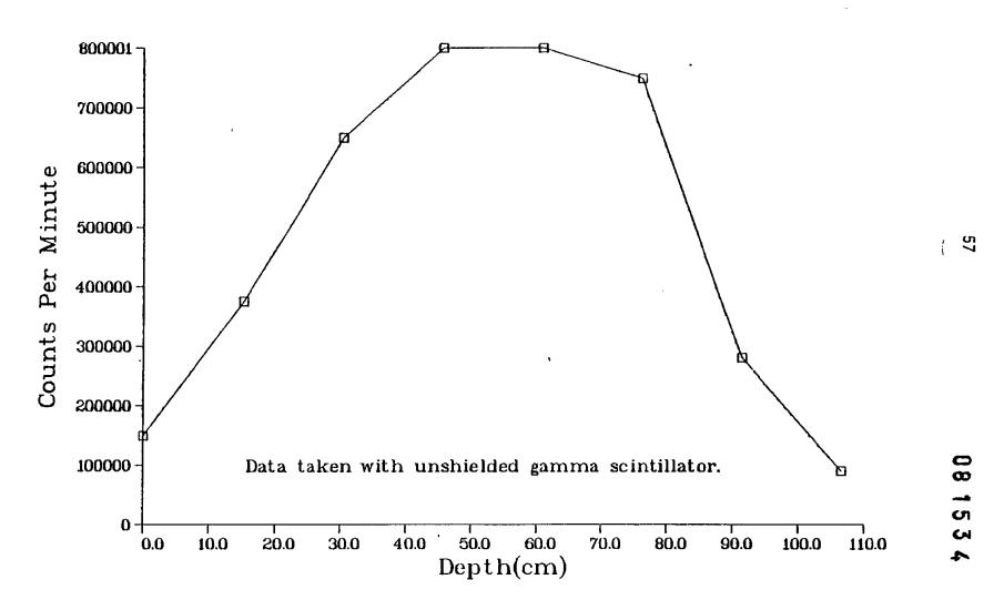
Fig. II-14. Gamma profile of core hole MJC32 (see Fig. 8)
