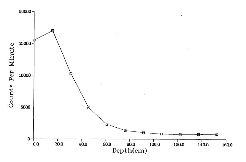
Fig. II-4. Gamma profile of core hole MJC22 (see Fig. 6)
