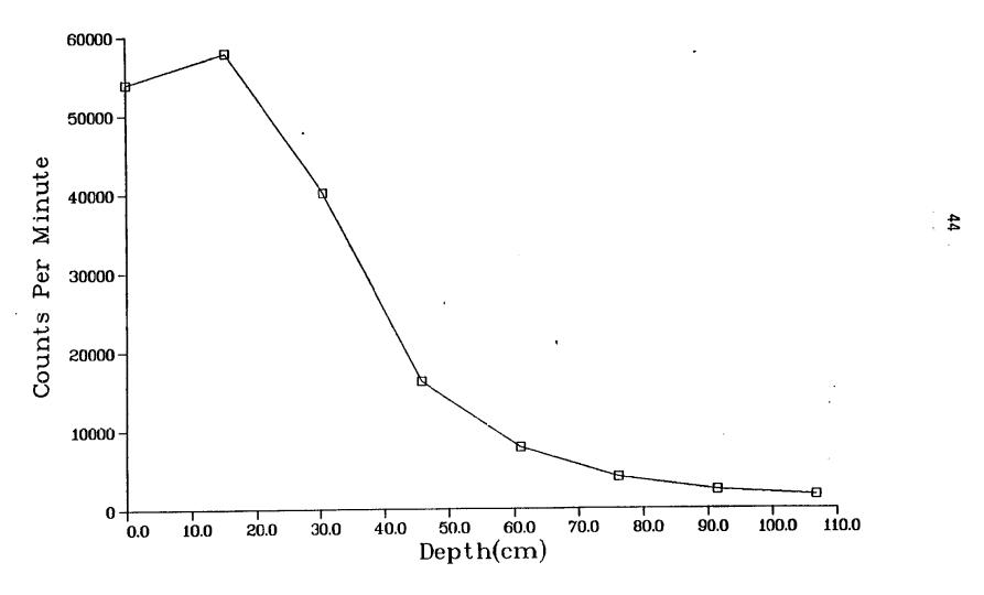
Fig. II-1. Gamma profile of core hole MJC19 (see Fig. 6)
