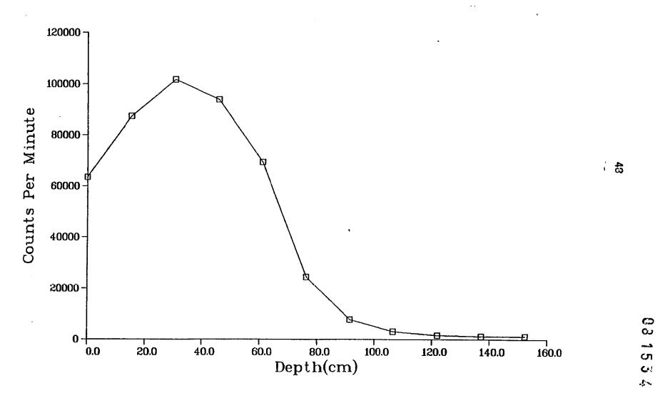
Fig. II-5. Gamma profile of core hole MJC23 (see Fig. 6)
