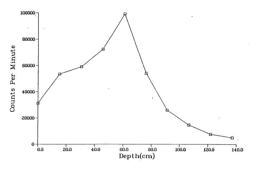
Fig. II-8. Gamma profile of core hole MJC26 (see Fig. 6)
