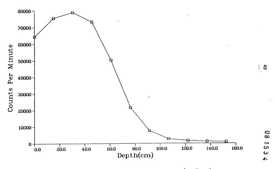
Fig. II-6. Gamma profile of core hole MJC24 (see Fig. 6)
