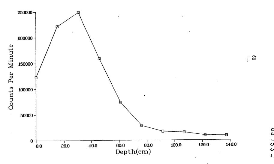
Fig. II-17. Gamma profile of core hole MJC45 (see Fig. 6)
