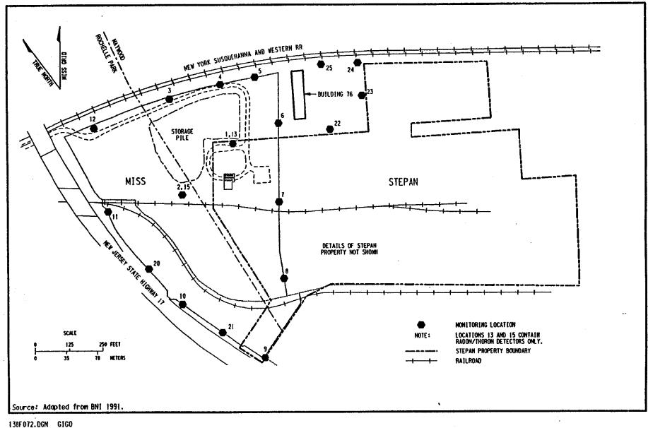
Figure 5-2 Onsite Radon, Thoron, and External Gamma Radiation Monitoring Locations
