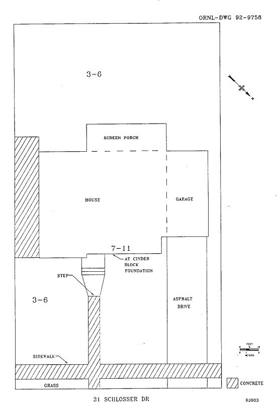
Fig. 1. Gamma radiation levels ( $\mu R/h$ ) measured on the surface at 31 Schlosser Drive, Rochelle Park, New Jersey (RJ003).
