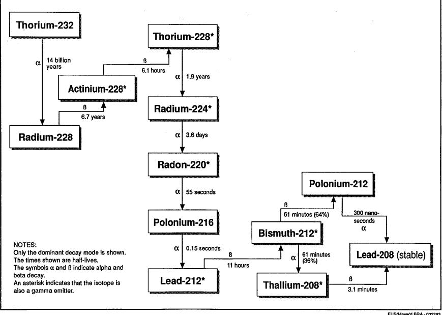
Figure 2-2. Thorium-232 Radioactive Decay Series
