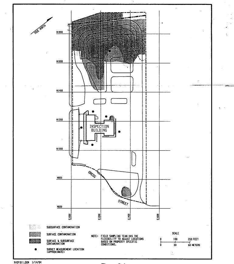
Figure 2-1 Areas of Contamination at the New Jersey Vehicle Inspection Station Property
