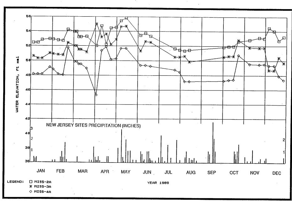
FIGURE 1-8 HYDROGRAPHS OF WELLS 2A, 3A, AND 4A IN THE UPPER GROUNDWATER SYSTEM AT MISS
