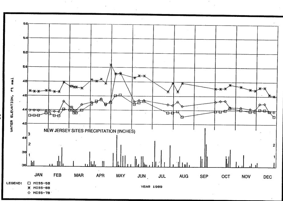
FIGURE 1-15 HYDROGRAPHS OF WELLS 5B, 6B, AND 7B IN THE BEDROCK GROUNDWATER SYSTEM AT MISS
