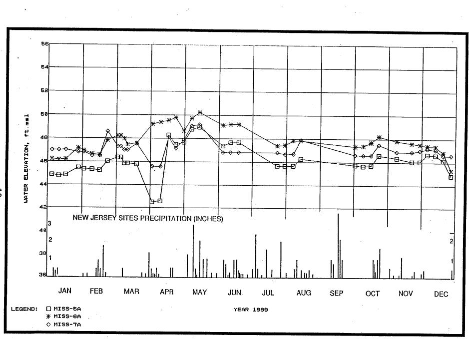
FIGURE 1-9 HYDROGRAPHS OF WELLS 5A, 6A, AND 7A IN THE UPPER GROUNDWATER SYSTEM AT MISS
