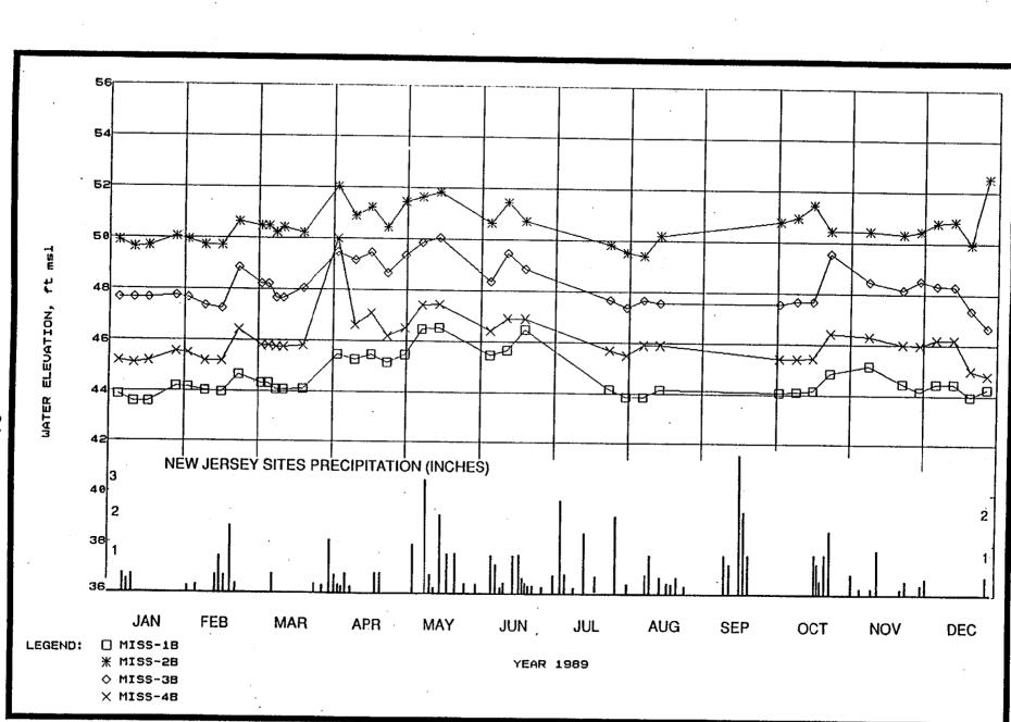
FIGURE 1-14 HYDROGRAPHS OF WELLS 1B, 2B, 3B, AND 4B IN THE BEDROCK GROUNDWATER SYSTEM AT MISS
