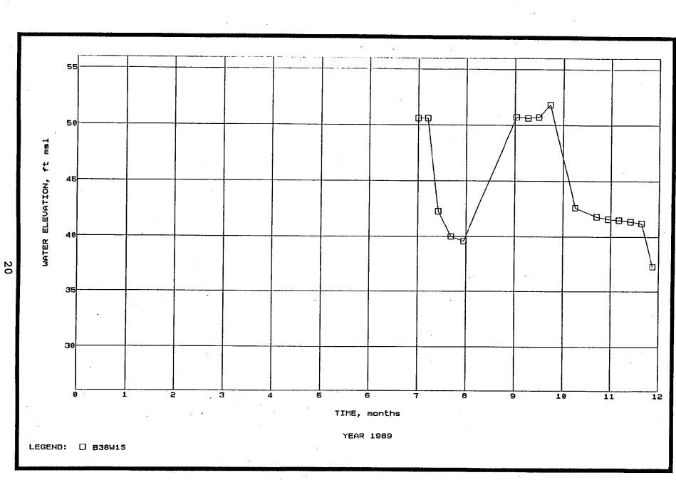
FIGURE 1-11 HYDROGRAPH OF WELL B38W10S IN THE UPPER GROUNDWATER SYSTEM AT MISS
