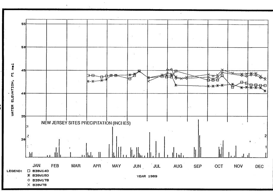
FIGURE 1-17 HYDROGRAPHS OF WELLS B38W14D, B38W15D, B38W17B, AND B38W07B IN THE BEDROCK GROUNDWATER SYSTEM AT MISS
