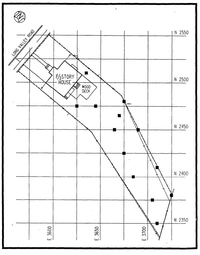
FIGURE 4-3 GAMMA EXPOSURE RATE MEASUREMENT LOCATIONS AT 14 LONG VALLEY ROAD
