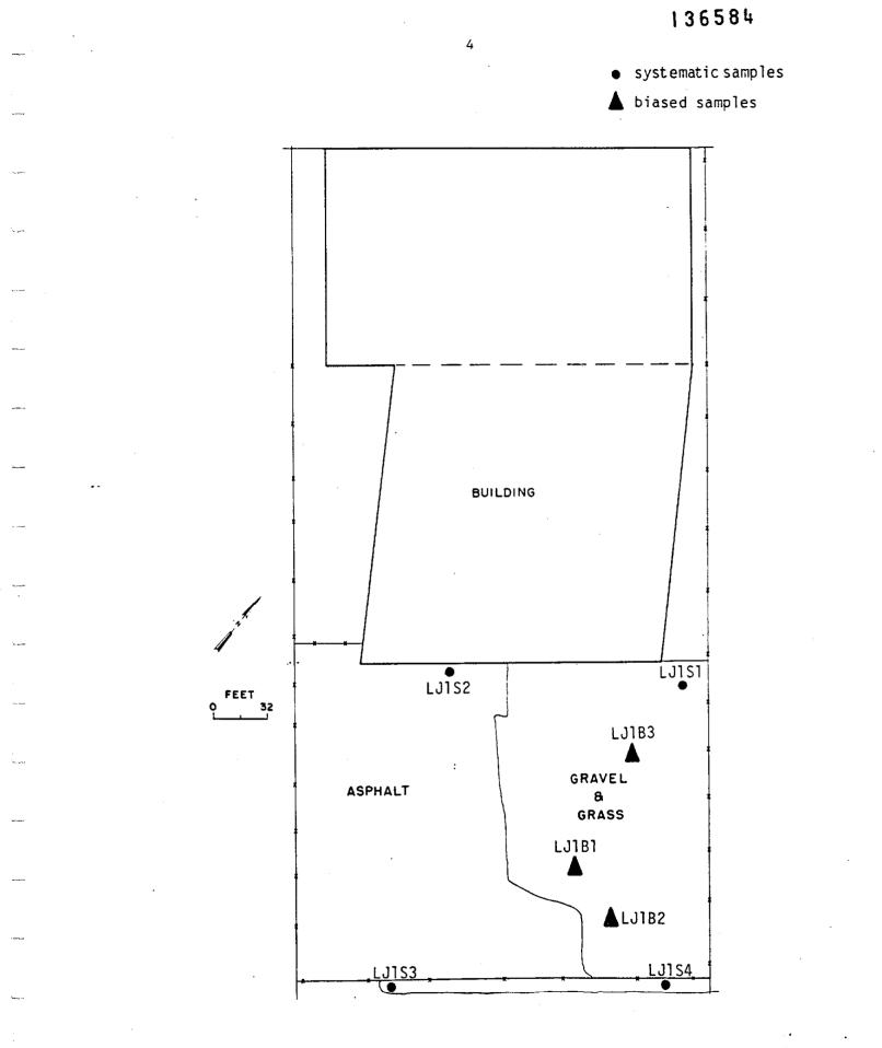
Fig. 1. Diagram showing locations of soil samples taken at 170 Gregg Street.
