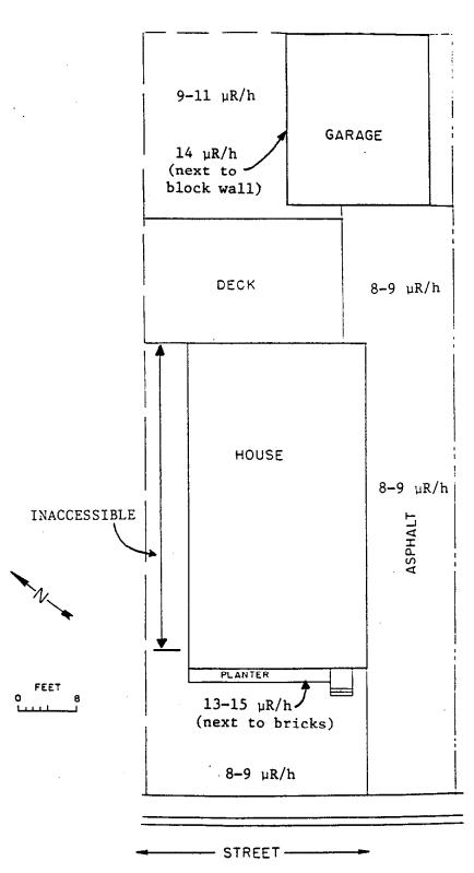
Fig. 2. Gamma radiation levels measured at 141 Washington Street, Lodi, New Jersey.
