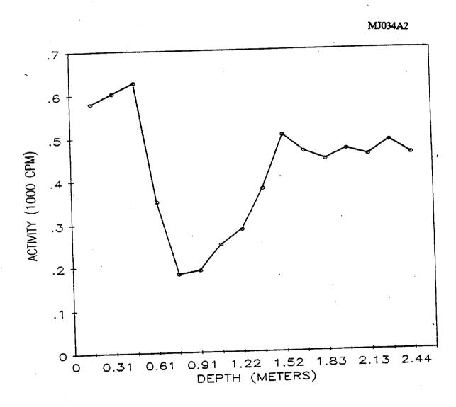
Fig. 4. Gamma profile of auger hole 2 at 146 West Central Avenue, Maywood, New Jersey.
