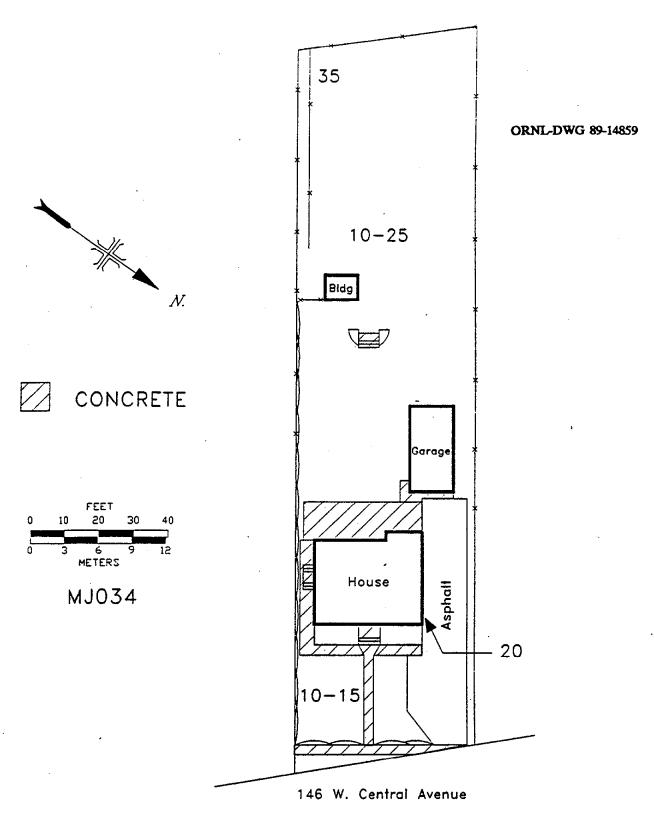
Fig. 1. Gamma radiation levels ( $\mu$ R/h) measured on the surface outdoors at 146 West Central Avenue, Maywood, New Jersey (MJ034).
