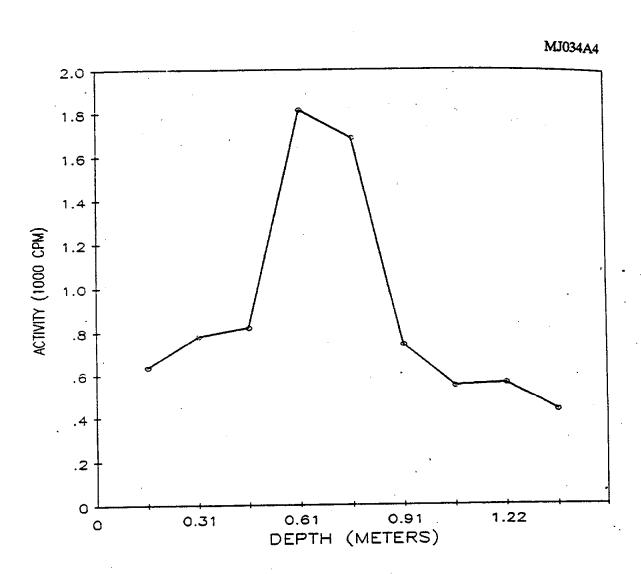
Fig. 6. Gamma profile of auger hole 4 at 146 West Central Avenue, Maywood, New Jersey.
