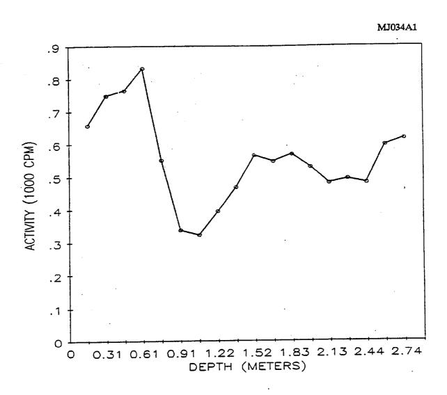
Fig. 3. Gamma profile of auger hole 1 at 146 West Central Avenue, Maywood, New Jersey.
