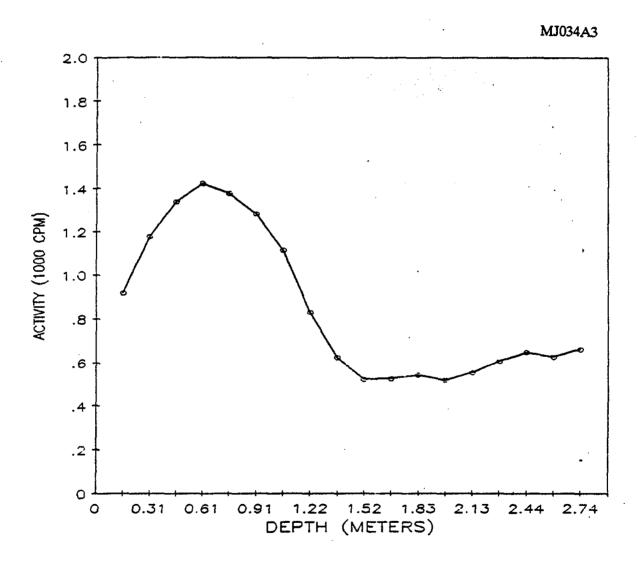
Fig. 5. Gamma profile of auger hole 3 at 146 West Central Avenue, Maywood, New Jersey.
