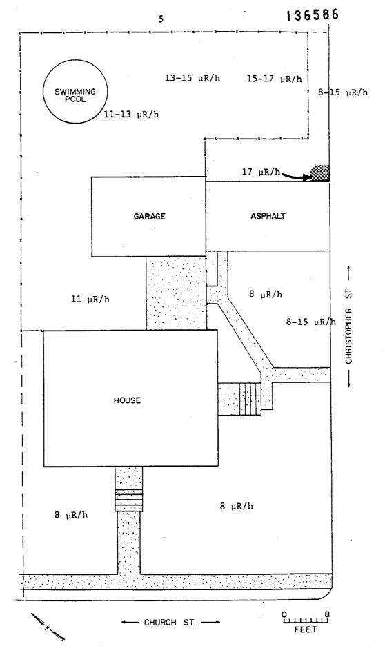
Fig. 2. Gamma radiation levels measured at 247 Church Street, Lodi, New Jersey.
