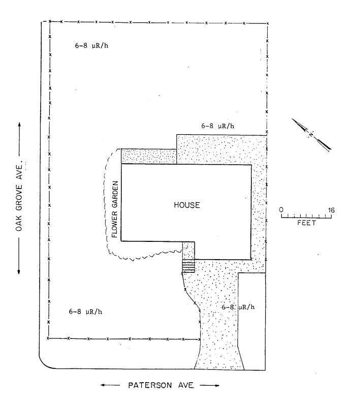
Fig. 2. Gamma radiation levels measured at 101 Paterson Avenue, Hasbrouck Heights, New Jersey.
