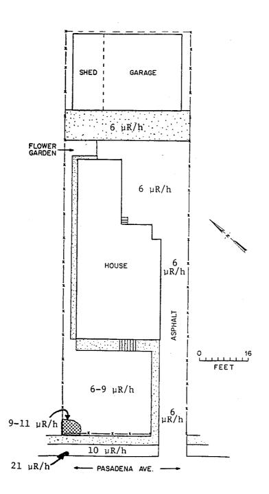
Fig. 2. Gamma radiation levels measured at 75 Pasadena Avenue, Lodi, New Jersey.
