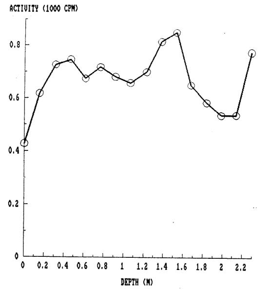
Fig. 4. Gamma profile for auger hole 2 (LJ056A2) at 19 Redstone Lane, Lodi, New Jersey.
