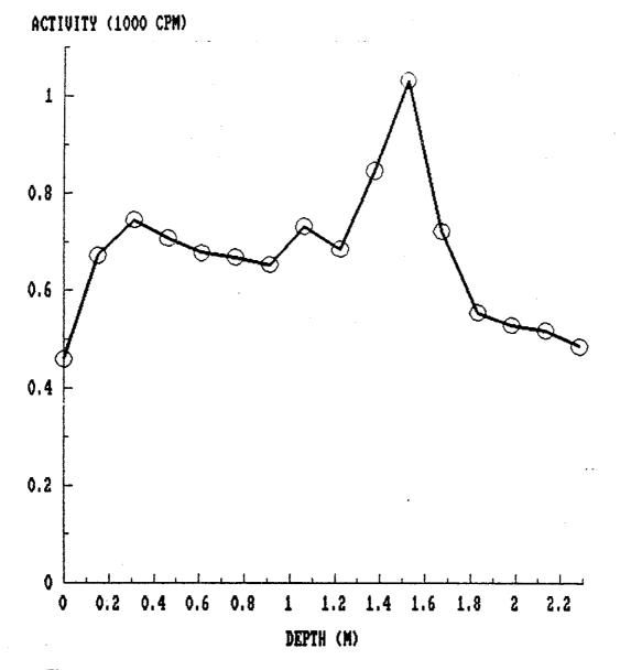
Fig. 3. Gamma profile for auger hole 1 (LJ056A1) at 19 Redstone Lane, Lodi, New Jersey.
