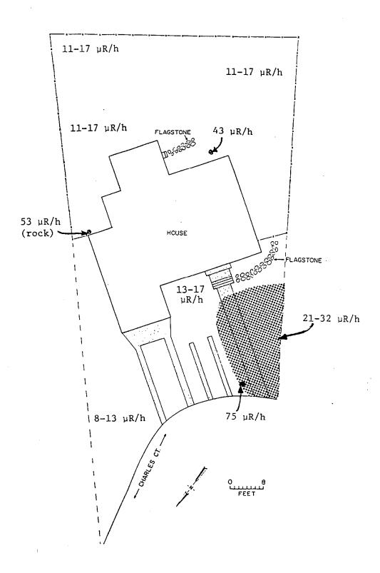
Fig. 2. Gamma radiation levels measured at 12 Charles Court, Lodi, New Jersey.
