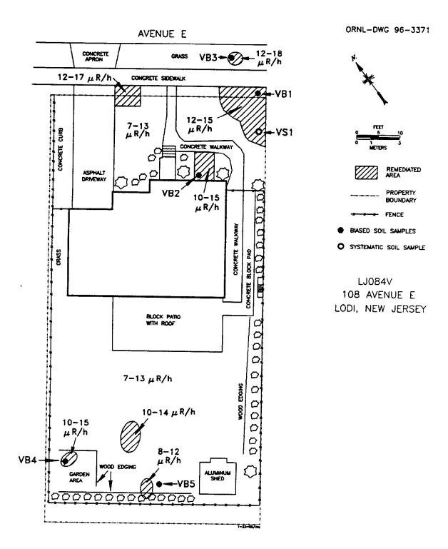
Fig. 2. Diagram showing gamma measurements and soil sampling locations at 108 Ave. E, Lodi, New Jersey.
