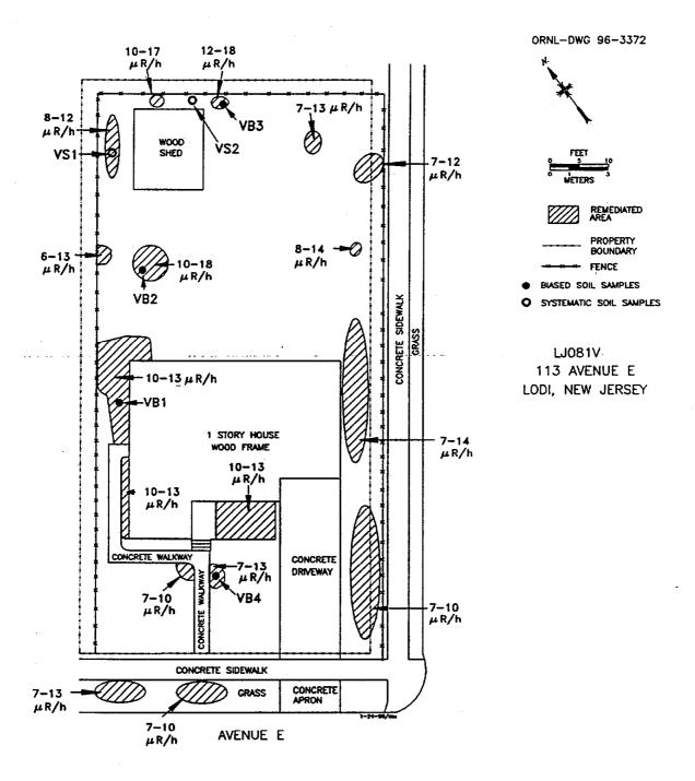
Fig. 2. Diagram showing gamma measurements and soil sampling locations at 113 Ave. E, Lodi, New Jersey.
