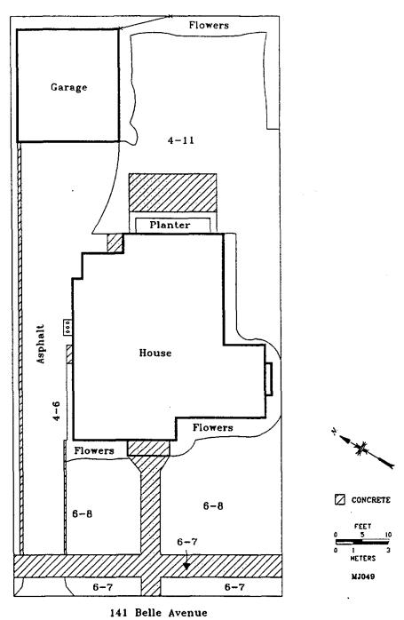
Fig. 1. Gamma radiation levels ( $\mu$ R/h) measured on the surface at 141 Belle Avenue, Maywood, New Jersey (MJ049).
