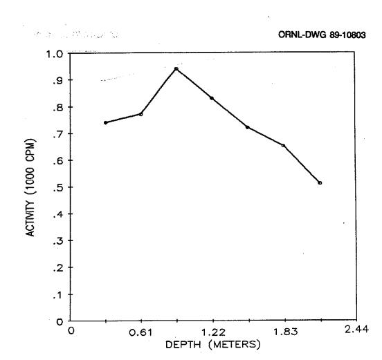
Fig. 3. Gamma profile for auger hole 1 (LJ042A1) at 9 Branca Court, Lodi, New Jersey.
