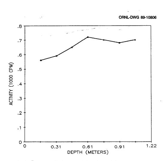
Fig. 6. Gamma profile for auger hole 4 (LJ042A4) at 9 Branca Court, Lodi, New Jersey.
