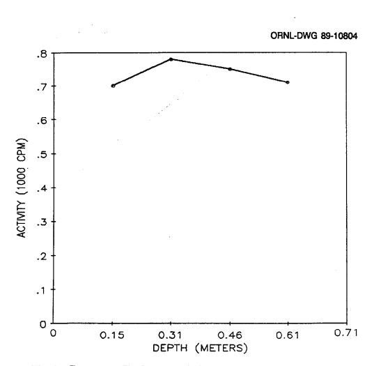
Fig. 4. Gamma profile for auger hole 2 (LJ042A2) at 9 Branca Court, Lodi, New Jersey.
