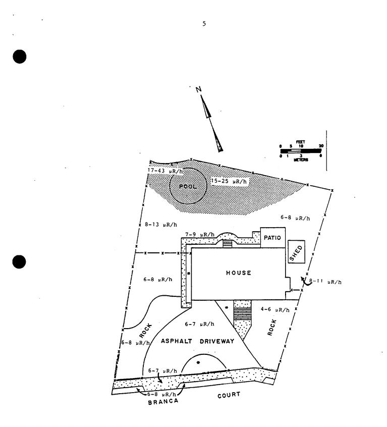
Fig. 2. Gamma radiation levels measured at 11 Branca Court, Lodi, New Jersey.
