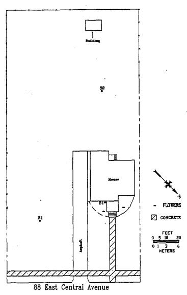
Fig. 2. Diagram showing locations of soil samples taken at 88 East Central Avenue, Maywood, New Jersey (MJ037).
