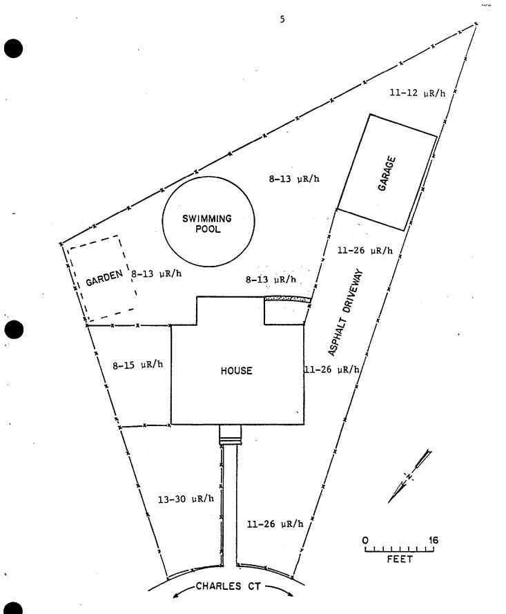
Fig. 2. Gamma radiation levels measured at 10 Charles Court, Lodi, New Jersey.
