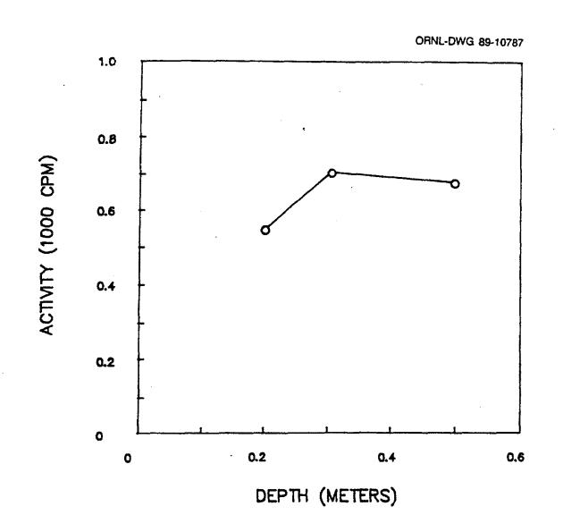
Fig. 10. Gamma profile for auger hole 9 (LJ045A9) at 30 Long Valley Road, Lodi, New Jersey.
