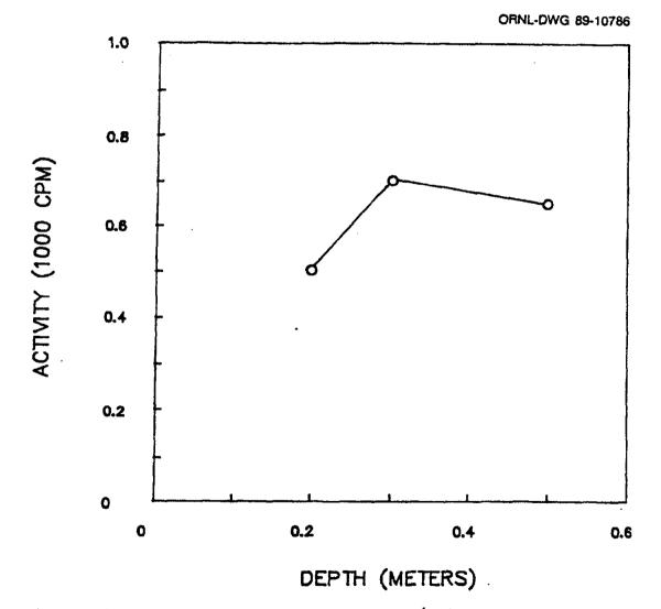
Fig. 9. Gamma profile for auger hole 8 (LJ045A8) at 30 Long Valley Road, Lodi, New Jersey.
