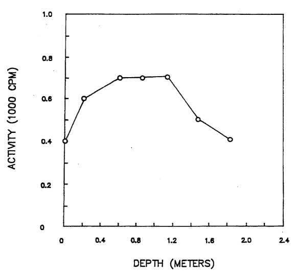
Fig. 5. Gamma profile for auger hole 3 (LJ045A3) at 30 Long Valley Road, Lodi, New Jersey.
