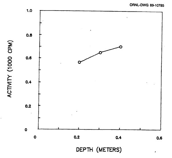
Fig. 8. Gamma profile for auger hole 7 (LJ045A7) at 30 Long Valley Road, Lodi, New Jersey.
