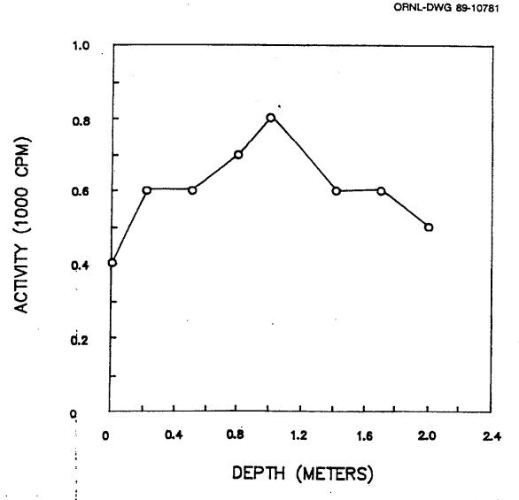
Fig. 4. Gamma profile for auger hole 2 (LJ045A2) at 30 Long Valley Road, Lodi, New Jersey.
