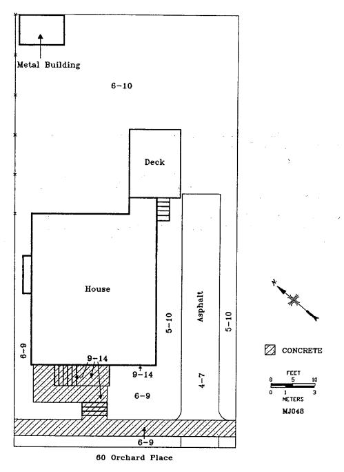
Fig. 1. Gamma radiation levels ( $\mu$ R/h) measured on the surface at 60 Orchard Place, Maywood, New Jersey (MJ048).
