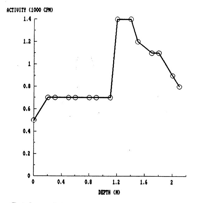
Fig. 4. Gamma profile for auger hole 2 (LJ028A2) at 9 Hancock Street, Lodi, New Jersey.
