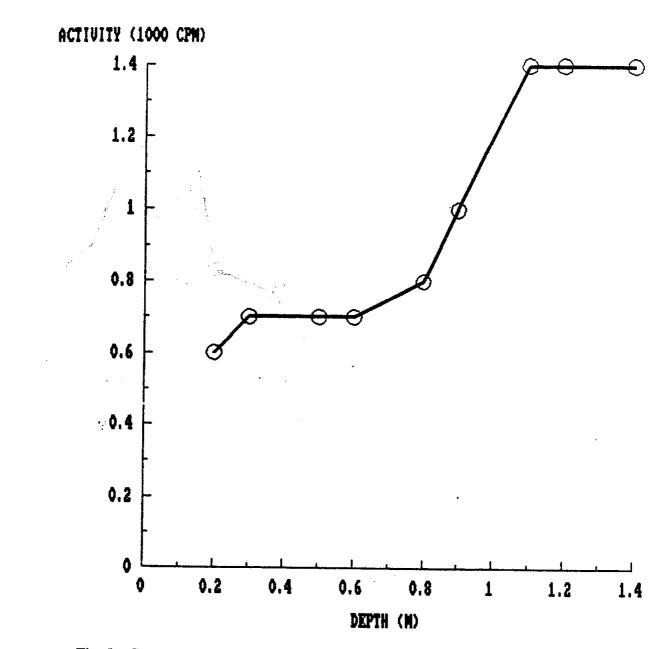
Fig. 5. Gamma profile for auger hole 3 (LJ028A3) at 9 Hancock Street, Lodi, New Jersey.
