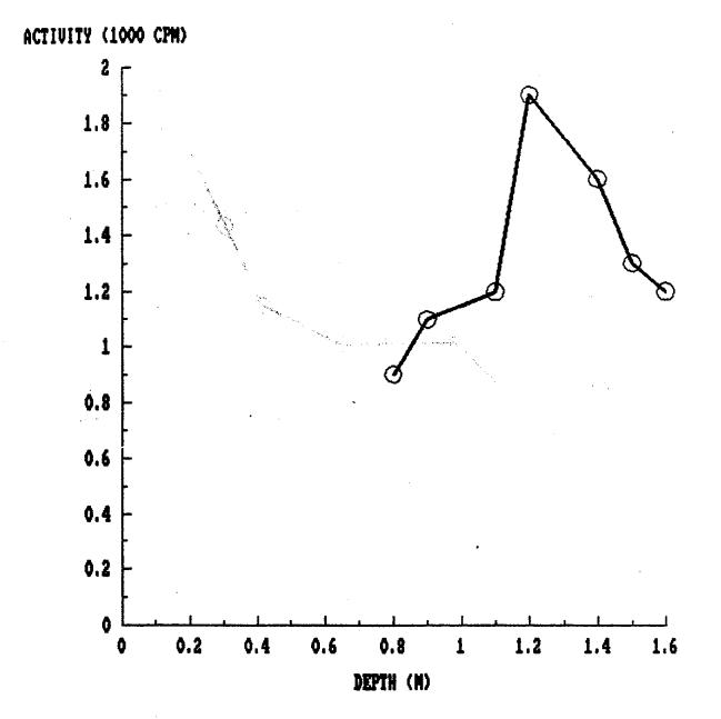
Fig. 6. Gamma profile for auger hole 4 (LJ028A4) at 9 Hancock Street, Lodi, New Jersey.
