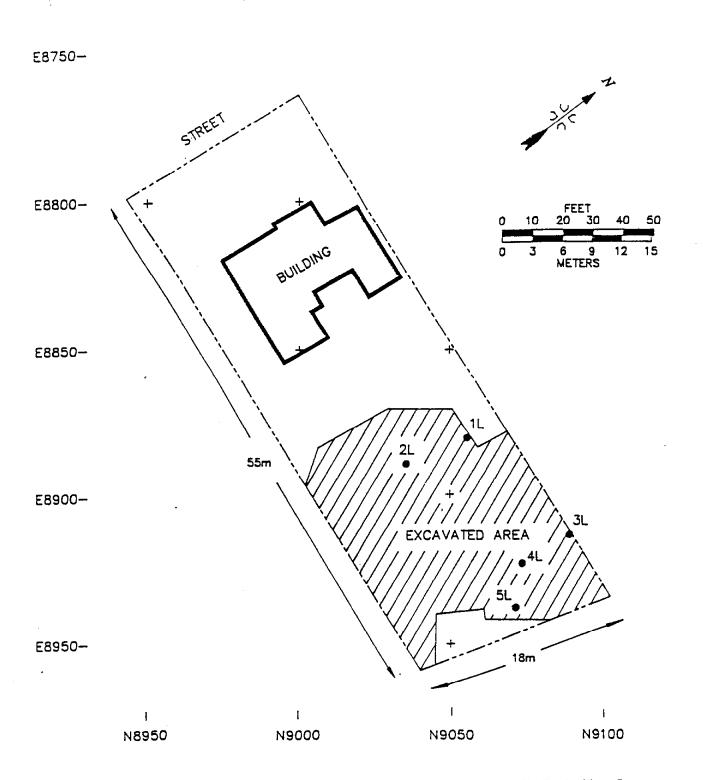
Fig 3. Locations of soil samples on the property at 90 Park Way, Rochelle Park, New Jersey (MJ01L).
