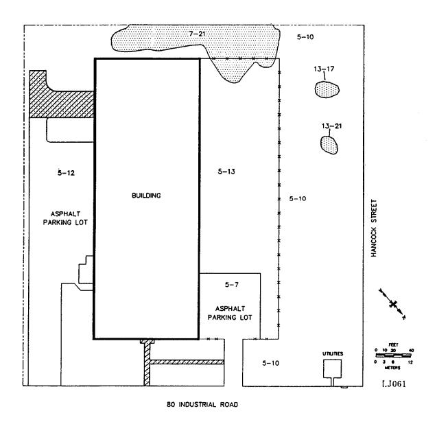
Fig. 1. Gamma radiation levels ( $\mu R/h$ ) measured on the surface at 80 Industrial Road, Lodi, New Jersey (LJ061).
