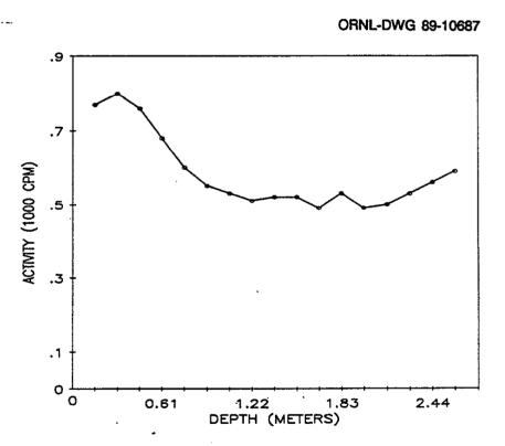
Fig. 6. Gamma profile for auger hole 5 (LJ061A5) at 80 Industrial Road, Lodi, New Jersey.
