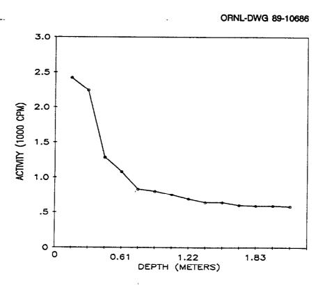
Fig. 5. Gamma profile for auger hole 4 (LJ061A4) at 80 Industrial Road, Lodi, New Jersey.
