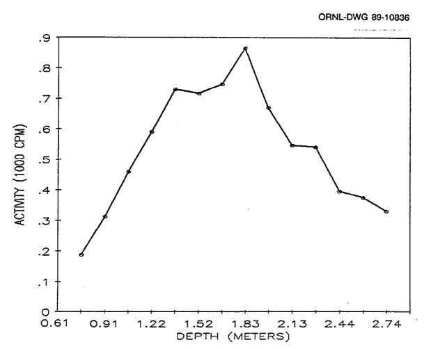
Fig. 7. Gamma profile for auger hole 5 (LJ076A5) at 199 Main Street, Lodi, New Jersey.
