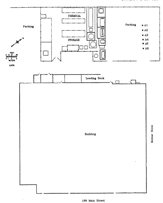
Fig. 2. Diagram showing locations of soil samples taken at 199 Main Street, Lodi, New Jersey (LJ076).
