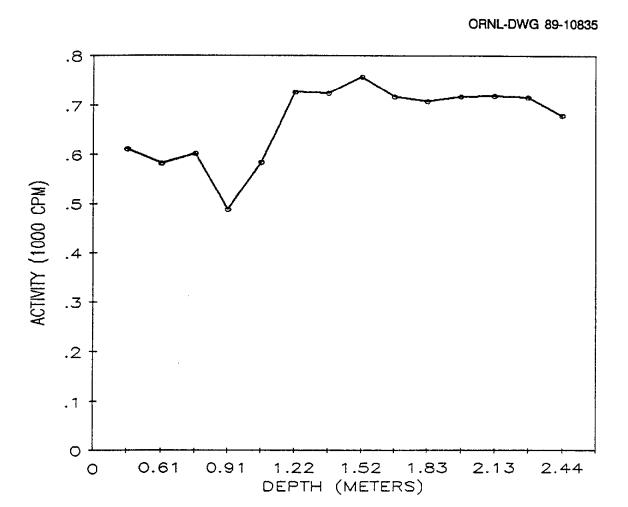
Fig. 6. Gamma profile for auger hole 4 (LJ076A4) at 199 Main Street, Lodi, New Jersey.
