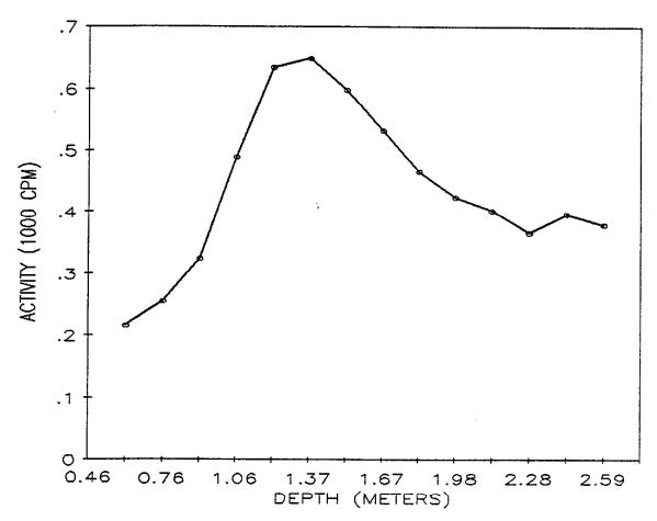
Fig. 4. Gamma profile for auger hole 2 (LJ076A2) at 199 Main Street, Lodi, New Jersey.
