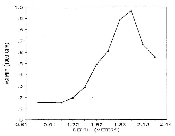
Fig. 8. Gamma profile for auger hole 6 (LJ076A6) at 199 Main Street, Lodi, New Jersey.
