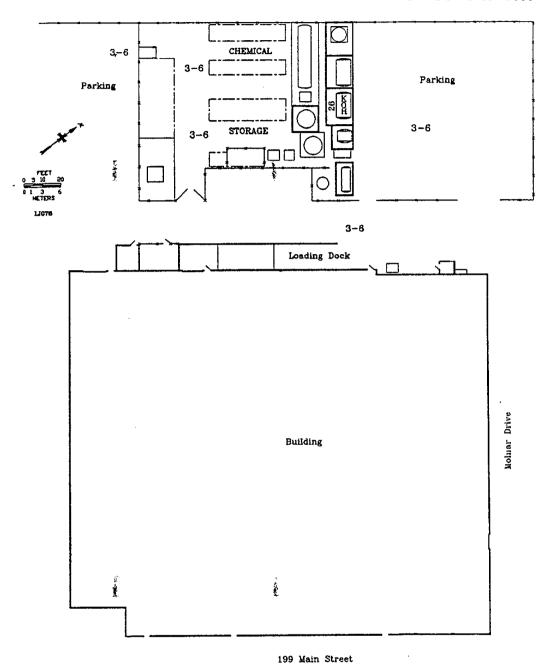
Fig. 1. Gamma radiation levels ( $\mu$ R/h) measured on the surface at 199 Main Street, Lodi, New Jersey (LJ076).
