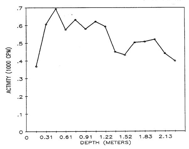
Fig. 5. Gamma profile for auger hole 3 (LJ076A3) at 199 Main Street, Lodi, New Jersey.
