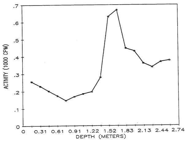
Fig. 3. Gamma profile for auger hole 1 (LJ076A1) at 199 Main Street, Lodi, New Jersey.
