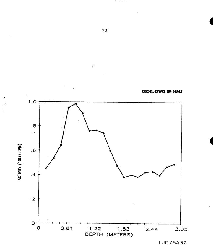
Fig. 17. Gamma profile for auger hole 32 at 205 Main Street, Lodi, New Jersey (LJ075).
