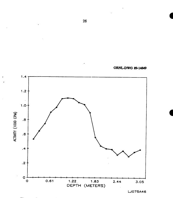
Fig. 21. Gamma profile for auger hole 46 at 205 Main Street, Lodi, New Jersey (LJ075).
