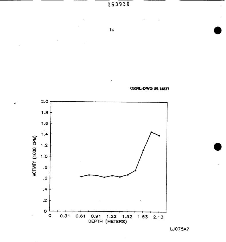
Fig. 9. Gamma profile for auger hole 7 at 205 Main Street, Lodi, New Jersey (LJ075).
