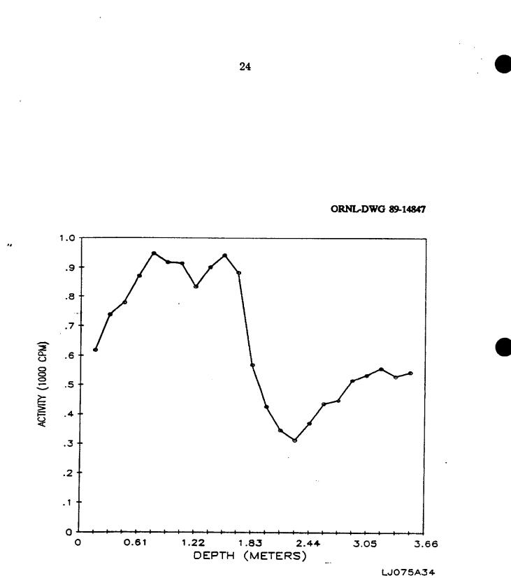
Fig. 19. Gamma profile for auger hole 34 at 205 Main Street, Lodi, New Jersey (LJ075).
