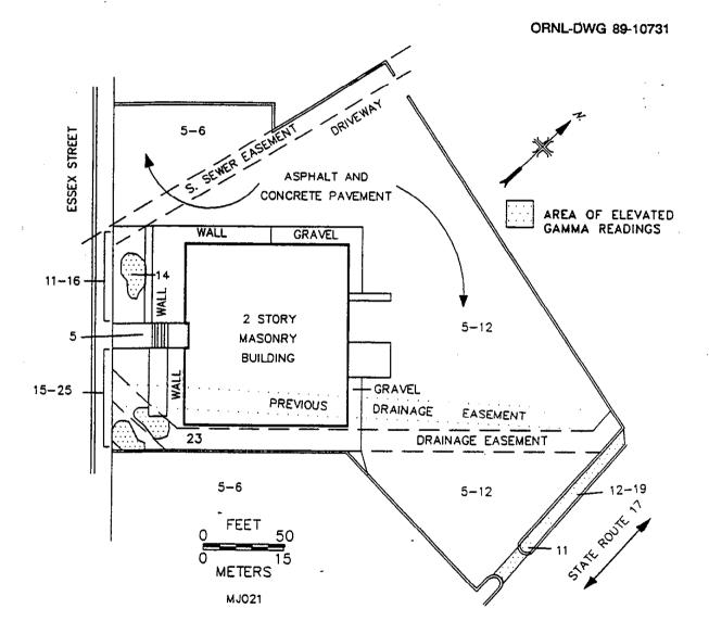
Fig. 1. Gamma radiation levels ( $\mu$ R/h) measured on the surface at the National Community Bank, 113 Essex Street, Maywood, New Jersey (MJ021).
