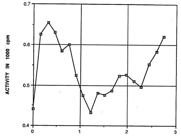
Fig. 5. Gamma profile for auger hole 3 (LJ093A3) at 72 State Highway 46, Lodi, New Jersey.
