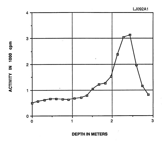
Fig. 3. Gamma profile for auger hole 1 (LJ092A1) at 80 State Highway 46, Lodi, New Jersey.
