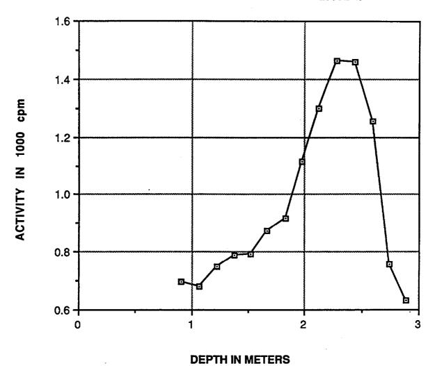
Fig. 5. Gamma profile for auger hole 3 (LJ092A3) at 80 State Highway 46, Lodi, New Jersey.
