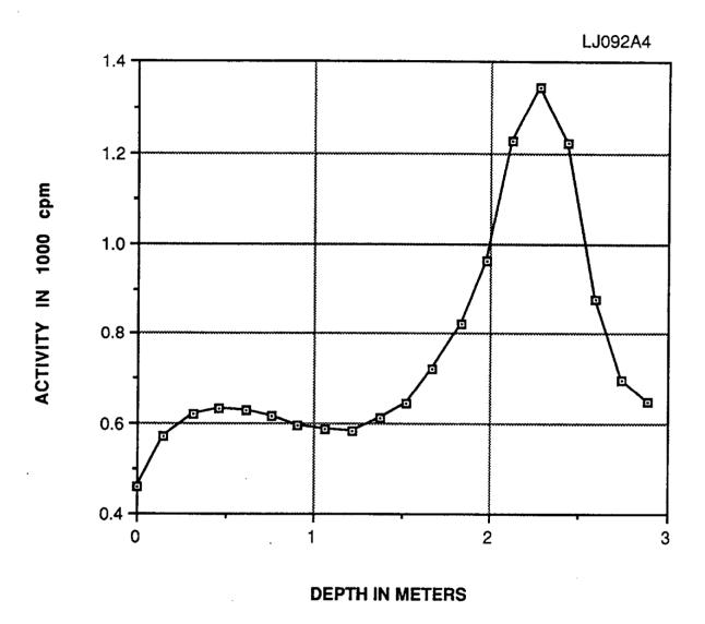
Fig. 6. Gamma profile for auger hole 4 (LJ092A4) at 80 State Highway 46, Lodi, New Jersey.
