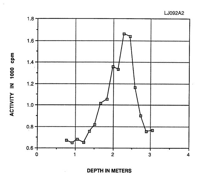
Fig. 4. Gamma profile for auger hole 2 (LJ092A2) at 80 State Highway 46, Lodi, New Jersey.
