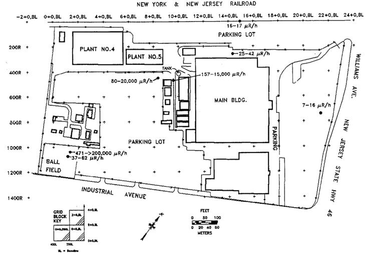
Fig. 2. Gamma radiation levels measured on the surface at Allied Bendix Aerospace Corporation, Industrial and Williams Avenues, Teterboro, New Jersey (TJ002).
