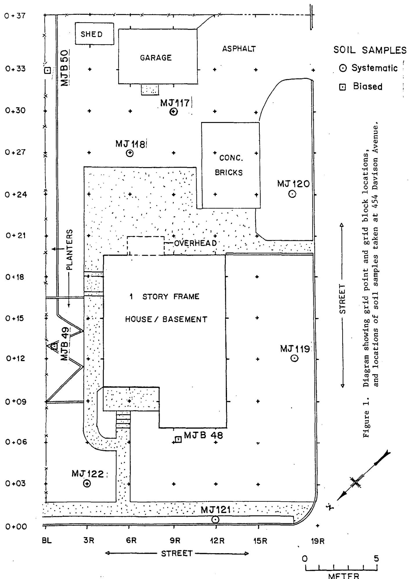
Figure 1. Diagram showing grid point and grid block locations, and locations of soil samples taken at 454 Davison Avenue.
